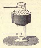
the jar, so as to indicate the temperatures of the upper and lower stratum of water.
